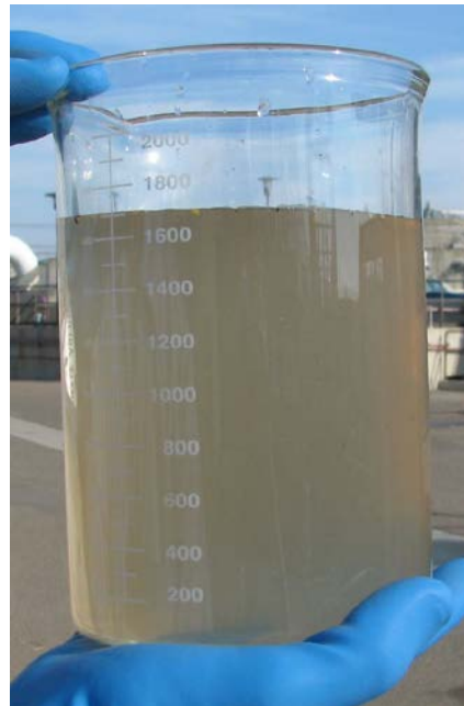
Primary Treated Effluent
