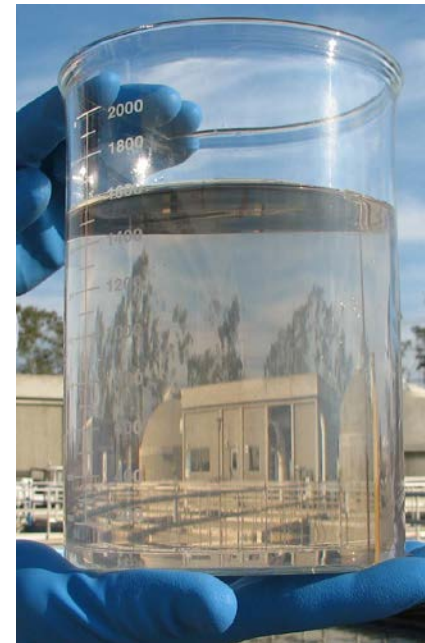
Secondary Treated Effluent
